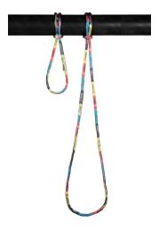
Compact Slings are excellent anchor slings and safety lanyards for rescue and rope access. Strong, durable, and easy to use, they are rated for a four-person load with a 100 kN MBS (end to end configuration). The High Tenacity Polyester (HTP) fiber core makes the Compact Sling highly durable and robust. An elastic polyester sleeve surrounds the internal load bearing elements for added protection, compact sizing, and easy handling.
